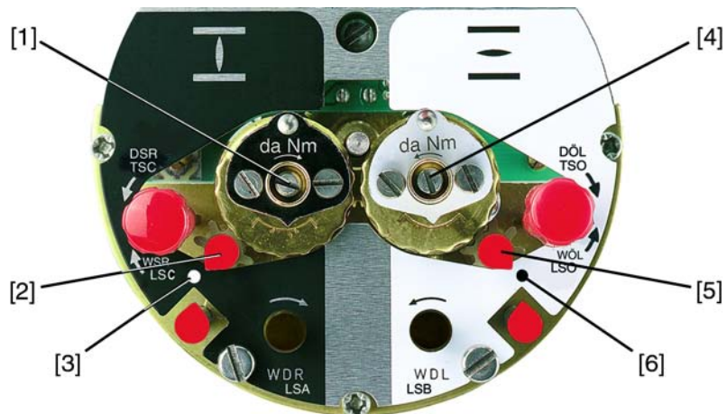
Figure 24: Setting elements for limit switching
