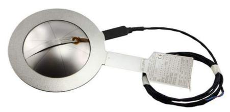
DonadonSDD IRA rupture sensors are simple and efficient instruments for recording the bursting of a rupture disc.
