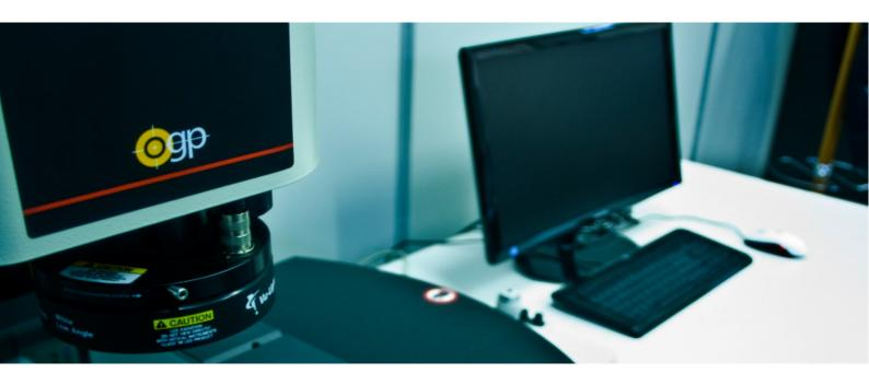
DonadonSDD has also invested in new up to date manufacturing equipment and modern development and measurement tools like Solidworks drawing equipment and an OGP microscope able to measure and take picture with 1 micron definition.
