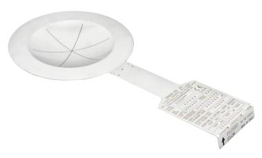
DonadonSDD SCR Rupture discs obtained with NS Nanoscored technology are compression or reverse discs with micro-scored calibrated sections opening in petals, characterised by the presence of 4, 6 or more radial scoring.
