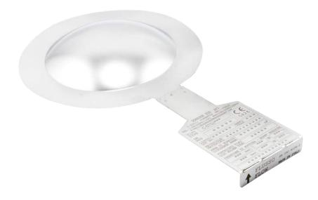
DonadonSDD STD rupture discs are conventional concave solid discs. This is a simple and reliable system used with gas and liquids in cyclic and pulsating pressure conditions. SCS discs react to excessive pressure in a few milliseconds. Supports may be provided for vacuum or counter-pressure protection.
