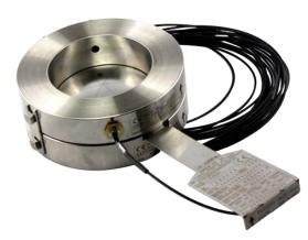
Optical rupture indicators Donadon OFI 04 and OFI 07 are very simple and reliable instruments for detecting bursting of discs. The terminals of the optical fibres are installed in the disc holder in a suitable position and are connected to an amplifier. Light transmission between the two optical fibres is interrupted by the bursting of the disc and a signal is sent to the plant's safety system.
