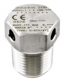
DonadonSDD SU/T sealed units are formed by a threaded connector containing a calibrated rupture disc. The rupture disc is welded to the connector. These units have been designed to make small disc mounting in plants easy and reliable, to simplify handling without need of specialised personnel.
