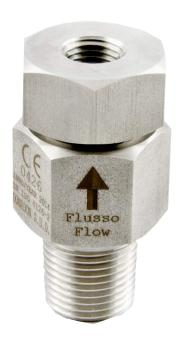
DonadonSDD SU/M sealed units are formed by a threaded connector, formed by two pieces, containing a calibrated rupture disc. The rupture disc is inserted in the threaded and sealed container. These units have been designed to make small disc mounting in plants easy and reliable, to simplify handling without need of specialised personnel.
