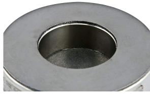
Disc material is high purity graphite. Opening is total but with fragmentation. Vacuum support is required for rupture pressures below 1.7 barg. Discs are self-supporting at higher calibrations.
