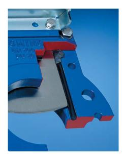
**Bidirectional shutoff** is achieved by the lateral gate surfaces and the elastic seat which is integrated in the body.
